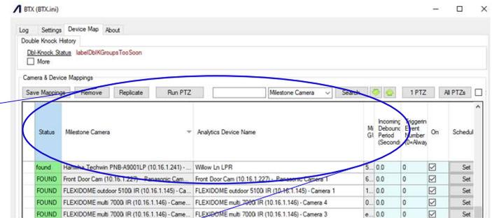
6. BTX generates an XProtect alarm record with video bookmark AND triggers rules and other security actions appropriate for a given list.
